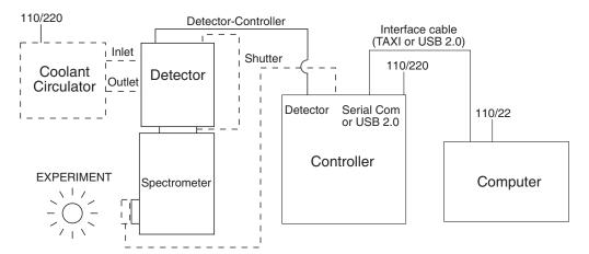
Figure 8. System Connection Diagram (TE Camera and Spectrometer)
